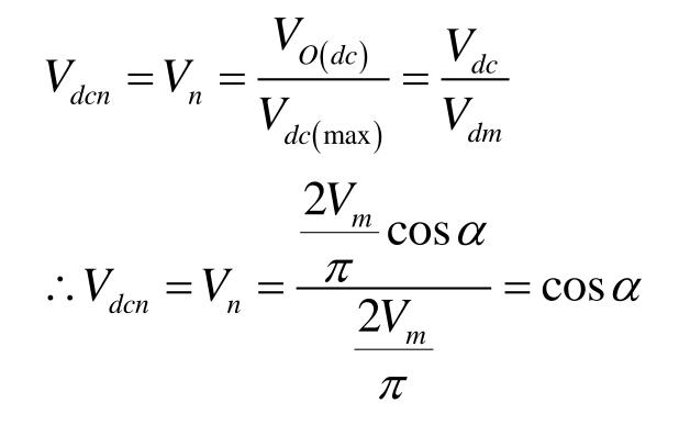
By plotting V<sub>O(dc)</sub> versus α, we obtain the control characteristic of a single phase full wave fully controlled bridge converter (single phase full converter) for constant & continuous load current operation. To plot the control characteristic of a Single Phase Full Converter for constant & continuous load current operation. We use the equation for the average/ dc output voltage
