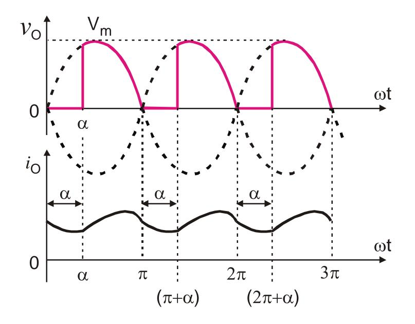
To Derive an Expression For The DC Output Voltage of Α Single Phase Semi-Converter With R,L, & E Load & FWD For Continuous, Ripple Free Load **Current Operation**
